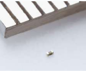
0201 size (0.25mmx0.125mm) ultra-small multilayer ceramic capacitors
